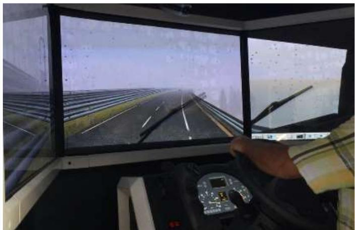
SITUATIONS FACED BY THE DRIVER IN THE SIMULATOR: INTERACTION WITH OTHER VEHICLES, JOINING TRAFFIC, FOG, RAIN, ETC.
